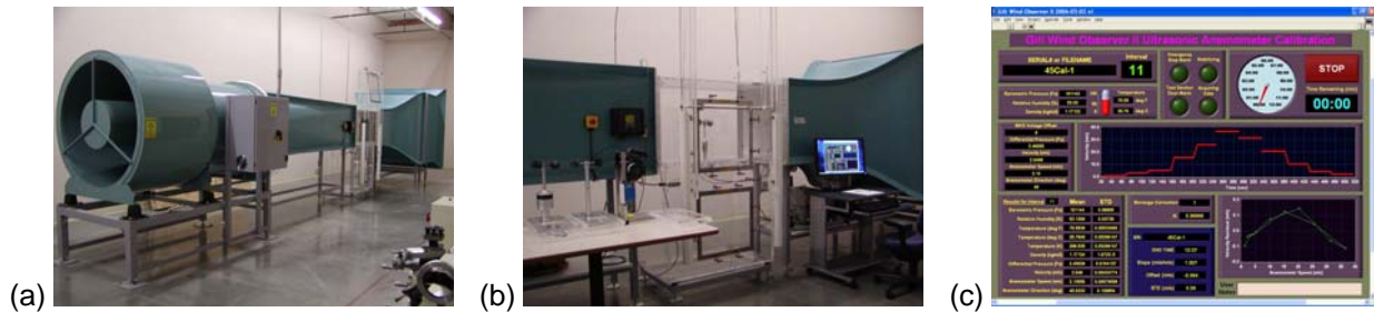
Figure 2: Otech Engineering Wind Tunnel Laboratory, WT3A: (a) Overall view, (b) Close-up view of test section, and (c) Sample LabVIEW front panel display.
