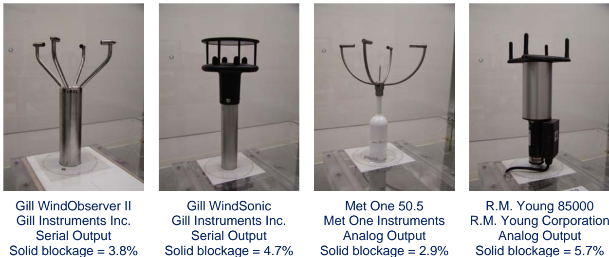
Figure 1: Sonic anemometer models tested in Otech Wind Tunnel, WT3A.
