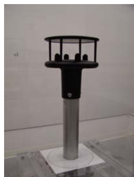
Gill WindSonic Gill Instruments Inc. Serial Output Solid blockage = 4.7%
