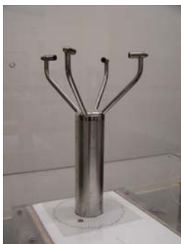
Gill WindObserver II Gill Instruments Inc. Serial Output Solid blockage = 3.8%
