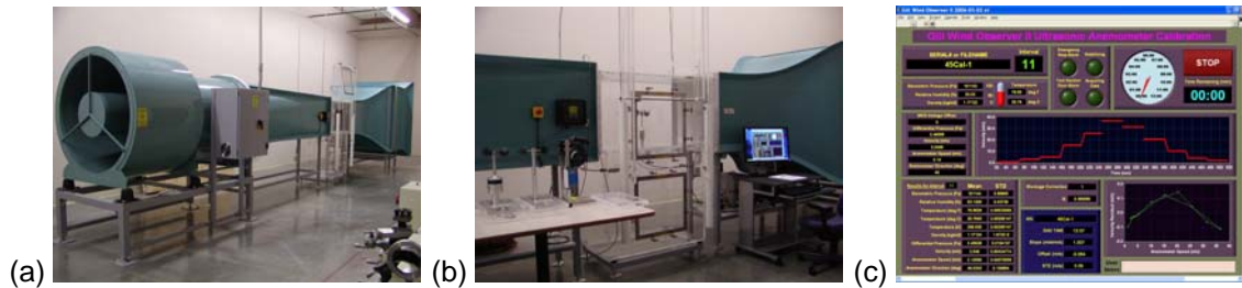
Figure 2: Otech Engineering Wind Tunnel Laboratory, WT3A: (a) Overall view, (b) Close-up view of test section, and (c) Sample LabVIEW front panel display.
